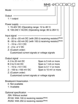
Note: Specify "/R100" or "/R250" when using different receiving resistor from the receiving resistor specified in the input signal suffix code "A" or "B".
