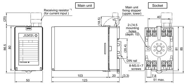
\*1: "250  $\Omega$ " or "100  $\Omega$ " is attached for current input.
